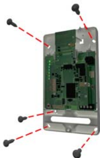
Figure 3: Mounting the Module
